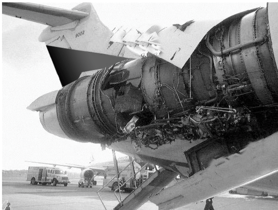
Figure III-12-22. Rupture du carter haute pression
